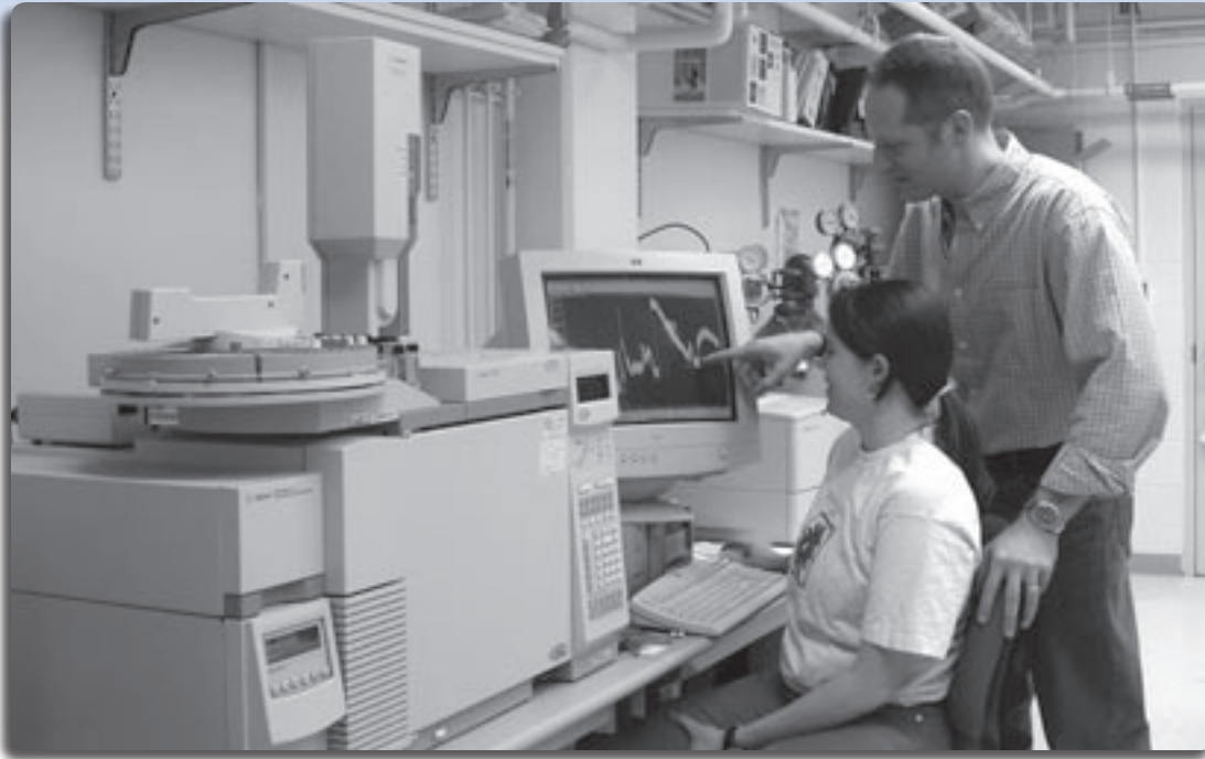
Dr. Horowitz and Lab Manager Amy Kaufman talk about isotope tracer data from a weight loss study using the gas chromatograph/mass spectrometer.
